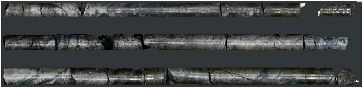
Photo 1 Scanned images of massive sulphide mineralization core, NB22-002: 337.1-340.2 m. Images are from within a broader interval of 18.27 m of 28.1% Zn, 0.65% Pb, and 68.4 g/t Ag.
