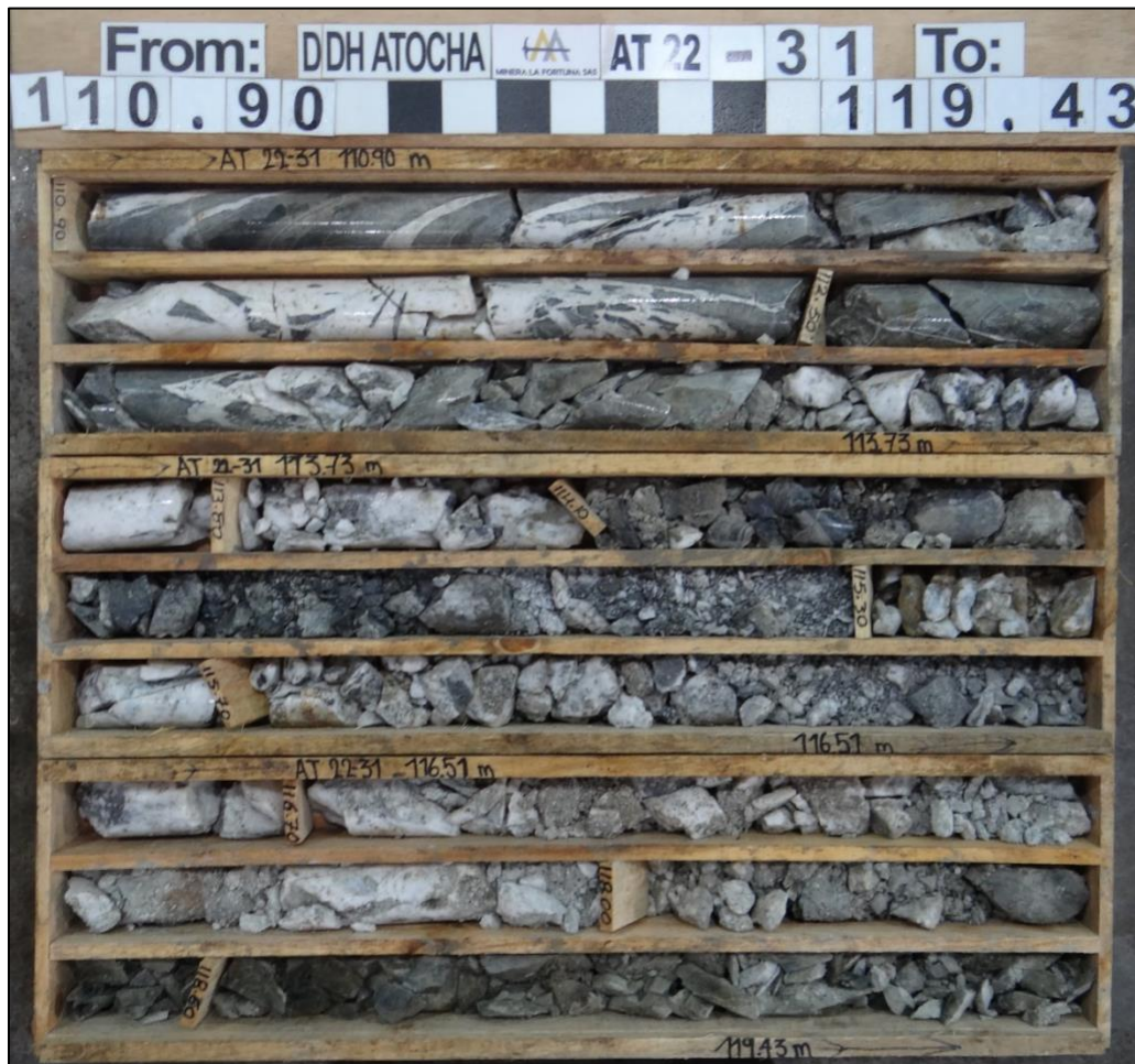
Photo 1. Wide (>7m) mineralized vein zone in hole AT-22-31 from 110.90 to 118.50m. Despite the impressive width of the interval, it was lacking the sulfide content and therefore precious metals values were also low.
