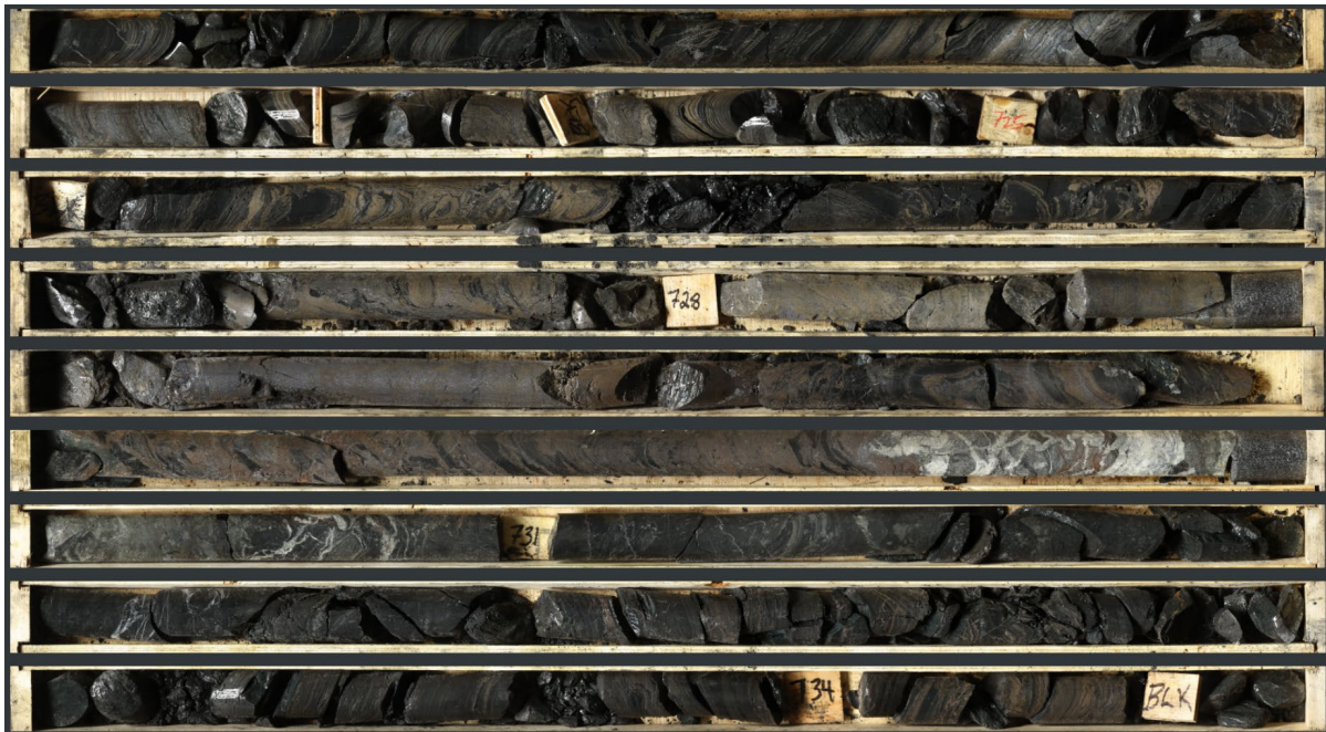
Photo 1: High resolution core scanning image of stratiform and massive to semi-massive sulphide mineralization in TS23-009 (722.4 m to 734.3 m)
