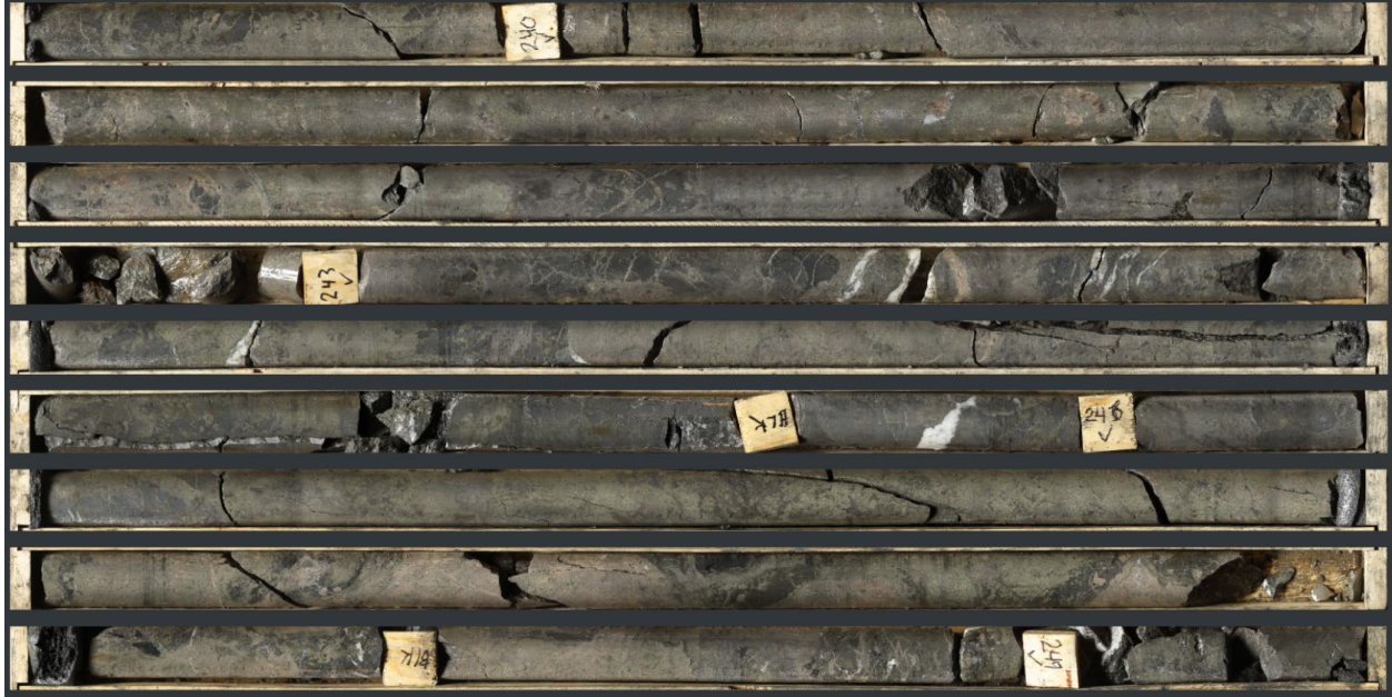
Photo 2: High resolution core scanning image of stratiform and massive to semi-massive sulphide mineralization in NB23-036 (239.6 m to 249.2 m)
