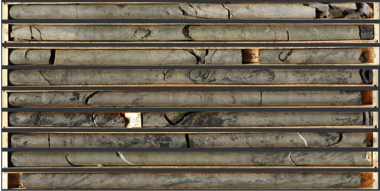
Photo 3: High resolution core scanning image of stratiform and massive to semi-massive sulphide mineralization in NB23-028 (330.2 m to 340.1 m)
