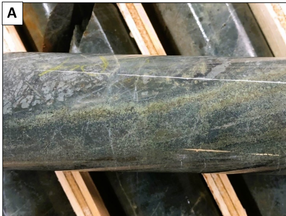
Figure 5: Examples of core from South Zone A) AXE-23-014: Fine disseminated pyrite-chalcopyrite-magnetite in brecciated intermediate volcanics and tuff beds at 740 m; B) AXE-23-012: Pyrite-chalcopyrite in quartz and as patches in altered volcanics with garnet at 372 m.
