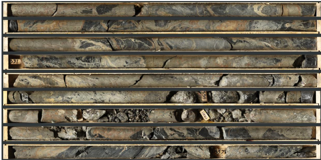
Photo 1: High resolution core scanning image of sphalerite-pyrite-siderite veins and semi-massive sulphide mineralization in NB23-008 (327.5 m to 337.2 m).
