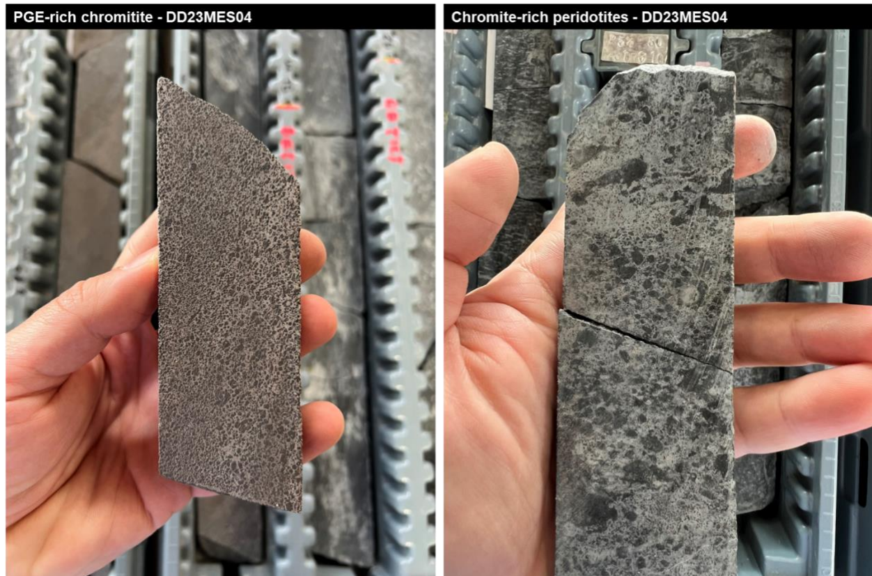
Figure 3: Core photographs of PGE-bearing chromitites and peridotites intersected at Salvador. Photo on the left showing a PGE-rich chromitite portion of the high-grade interval at DD23MES04 (10 m at 5.02 g/t 2PGE+Au from 88.65 m).
