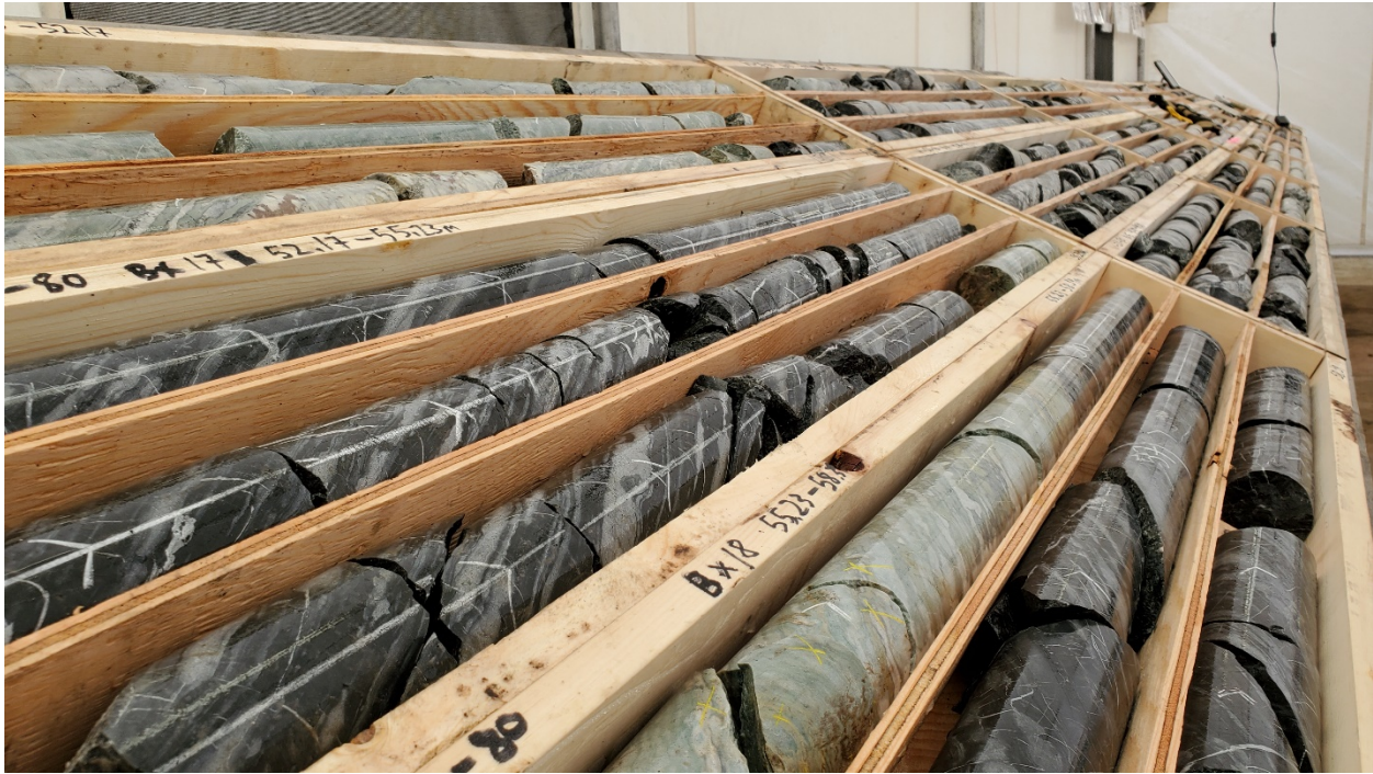
Image 2: Geotechnical Drill Core from Hole WI23-80 Wicheeda REE Deposit Open Pit Highwall
