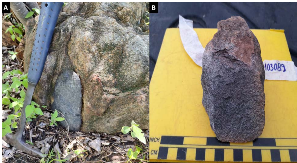
Figure 2: Photographs of high-grade outcrop and rock samples from Tróia target. A: Outcrop sample 103011 (12.00 g/t 2PGE+Au). B: Grab sample 103089 (23.01 g/t 2PGE+Au).
